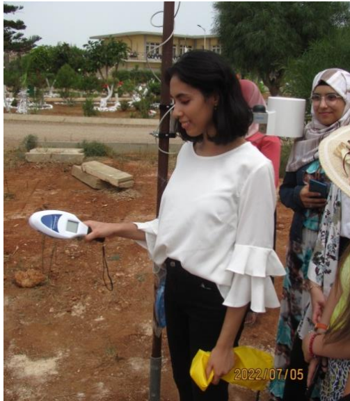
Much easier: GreenSeeker to measure how plants are growing.
